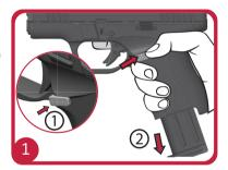
c. Lock the slide to the rear and check the chamber to make sure there is no ammunition inside the chamber. Double-check the chamber again to ensure there isn't any ammunition seated inside the chamber. (Figure 2)
